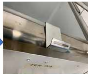
Bottom hinge part installation Place the bottom hinge on the SS top as shown in the picture above.
