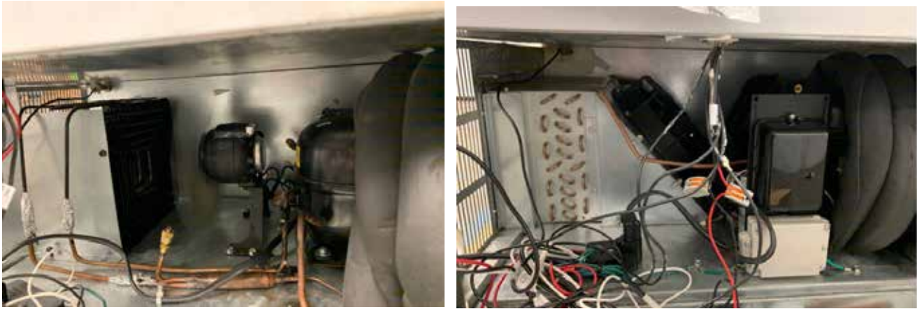
Hermetic Compressors, jelly roll & fin and tube condenser
