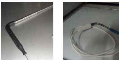
Figure 2: NTC Needle Probe Types
