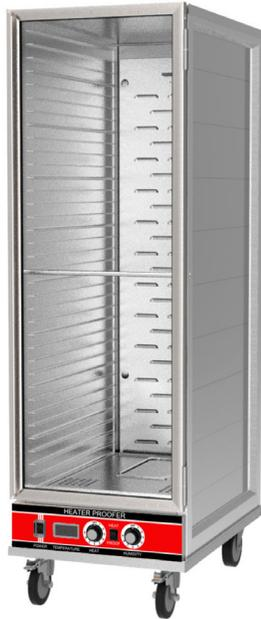
Keep food hot and proof dough with the Adcraft Full Size Heater Proofer. This non-insulated heater proofer is constructed of anodized 6063 aluminum extrusion with .08" thick aluminum base with formed channels. It has a field reversible door to accommodate any commercial kitchen space. This full-size heater proofer holds up to 36 full sheet pans with 1-1/2" clearance between slides. The door is made of durable 0.08" thick clear Lexan, which provides visibility without heat loss.
